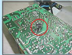
Spark trace. Electrical short circuit by rework or extraneous material are the reason.
