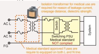
When power supply does not comply with the standards, customers are required to prepare for input fuses and insulating transformer etc. Because fuses and transformer will be installed separately, system will be large and expensive.
