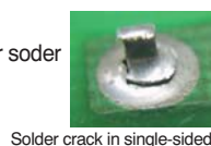
Solder crack in single-sided
