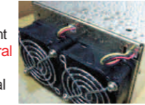
Under harsh neutral salt spray test
