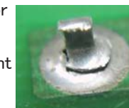
Solder crack (single-sided PWB)
