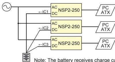
Note: The battery receives charge current of (IC1~IC3) 0.5±0.2A from each NSP2-250 power supply.
