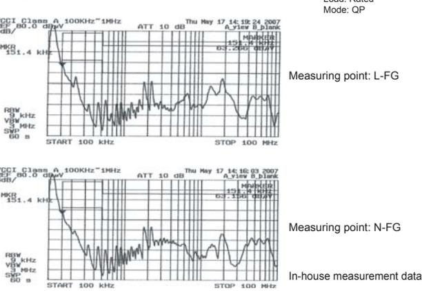
● Fig.8 Conducted Emission at 240 VAC
