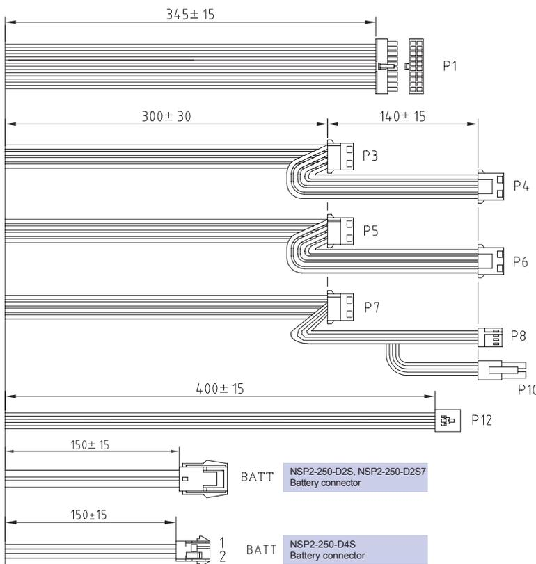
\*The battery connector for NSP2-250-D4P is mounted on the front panel.
