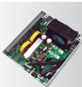
Internal Structure of Secondary Unit
