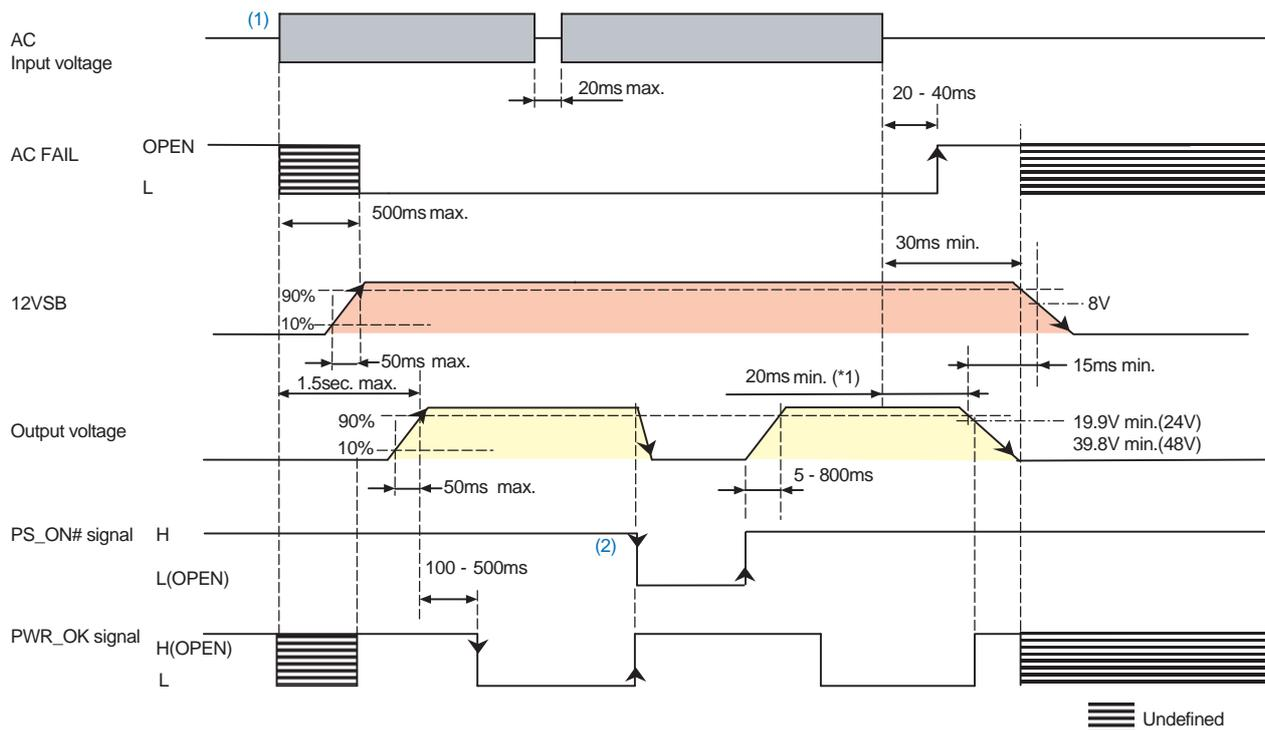
\*1 At 1000W output power. If it exceeds 1000W (lower than the continuous rated power), the period shall be 10ms min.
