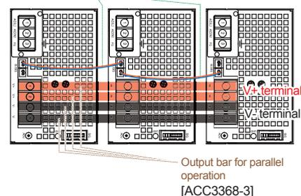
As in above picture, connect each output terminal with ACC3368-3 and each B.SIG terminal with WH-02XA02XA-150.
