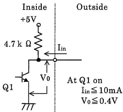
FAN\_C signal output circuit
