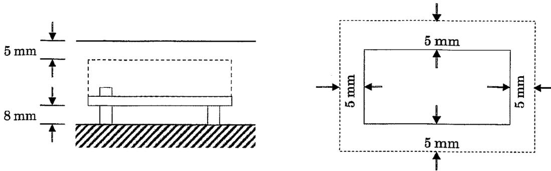
To suppress temperature rise around power supply, keep enough clearance to avoid poor convection.
