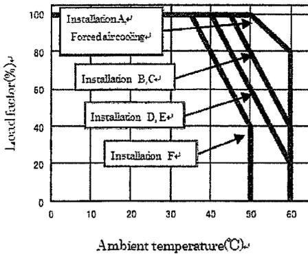
Figure 2. Derating curve for low input voltage
