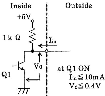
FAN\_M signal output circuit
