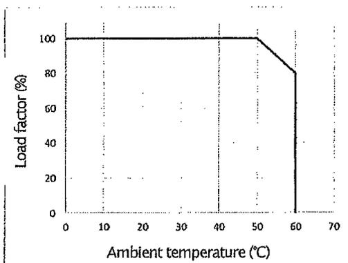
Figure 2. Low input voltage Derating chart
