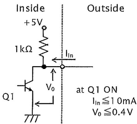
FAN\_M signal output circuit
