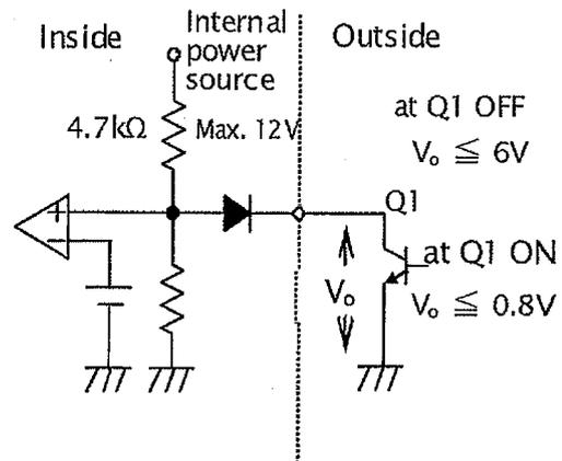
PWR\_OK signal output circuit
