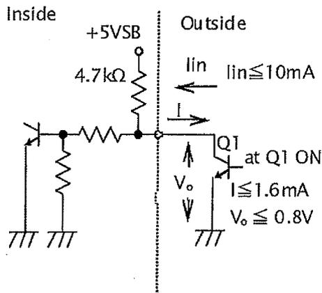
FAN\_C signal input circuit
