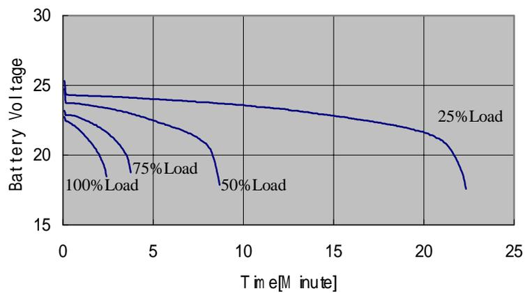
Battery : PS2538L(Lead-Acid Battery)
