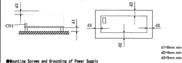
• Fix all 4 screws firmly at power supply mounting holes.
