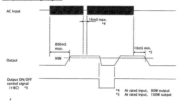
\*3 Model:UZP-120-\*\*-J\*L is equipped without the function of output ON/OFF control.
