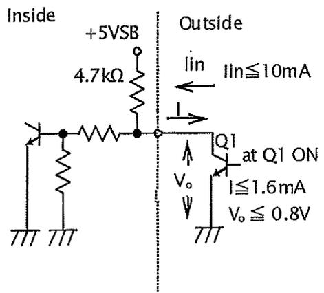
FAN\_C signal input circuit
