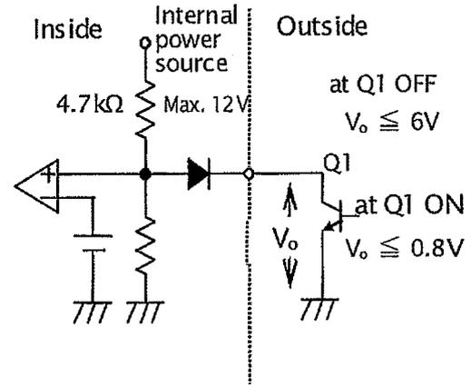
PWR\_OK signal output circuit
