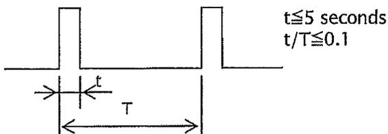
Figure 2. Definition of ripple and spike
