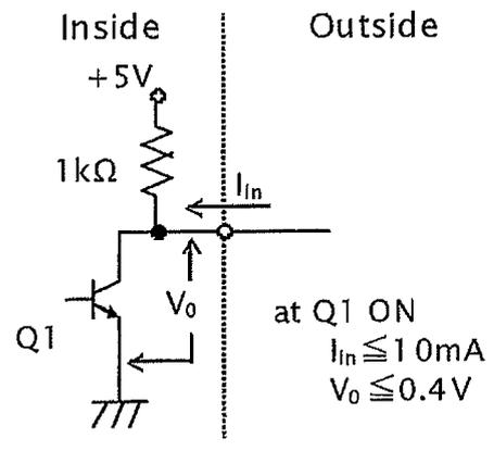
FAN M signal output circuit
