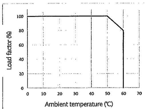
Figure 2. Low input voltage Derating chart
